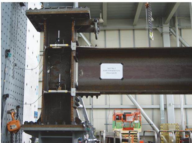
(b) Double split tee connection without a shear tab
