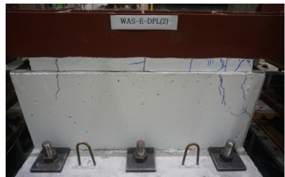
Fig. 9. Failure and crack patterns of specimens with the exterior-type indirect connection (WAS-E-DPL-T1)
