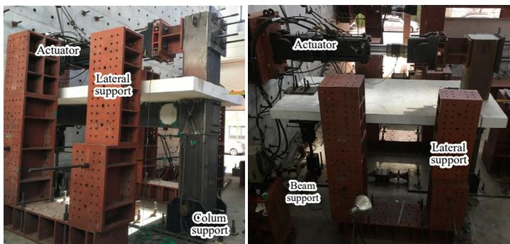
(a) Test setup for lateral loading of exterior beam-column connection
