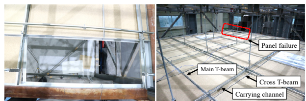
Fig. 16. Failure pattern of ITL specimen at the end of test
