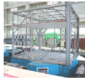
(b) Small-size test frame for triaxial shake table test
