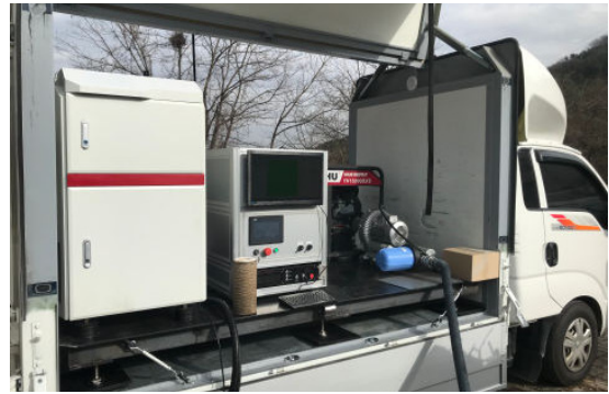
Fig. 2. Vehicle integrated clean laser system
