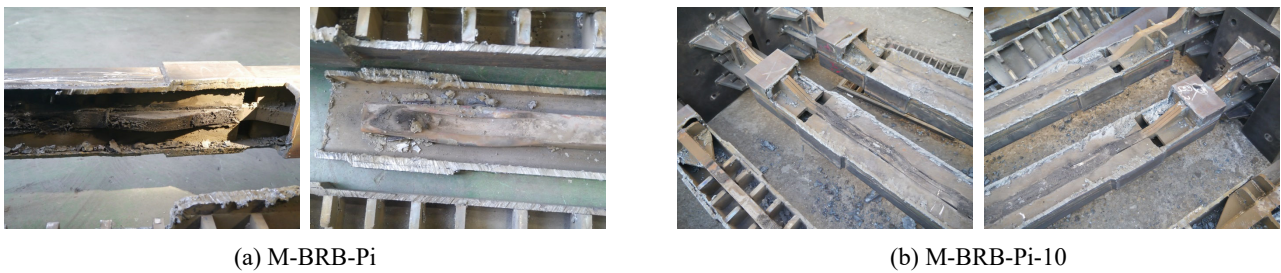
Fig. 9. Failure mode of each specimen
