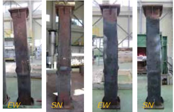
(a) Axial load: 5,000kN (b) Axial load: 2,500kN
