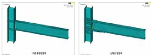
(a) Welded Connection (b) Proposed Connection
