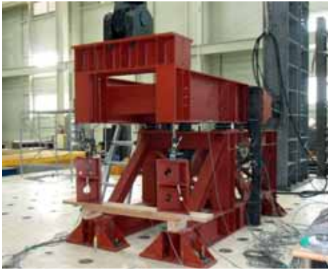
Fig. 14 Test Specimen of Rahman-type Movable Joint System
