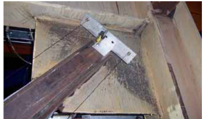
Fig. 12 Yielding in 2 nd floor west gusset plate
