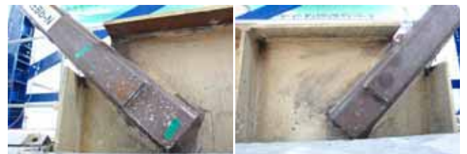
Fig. 13 Mild yielding in 2 nd floor mid-span gusset plate
