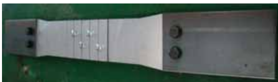
Fig. 7 Specimen connected to holding experiment tool
