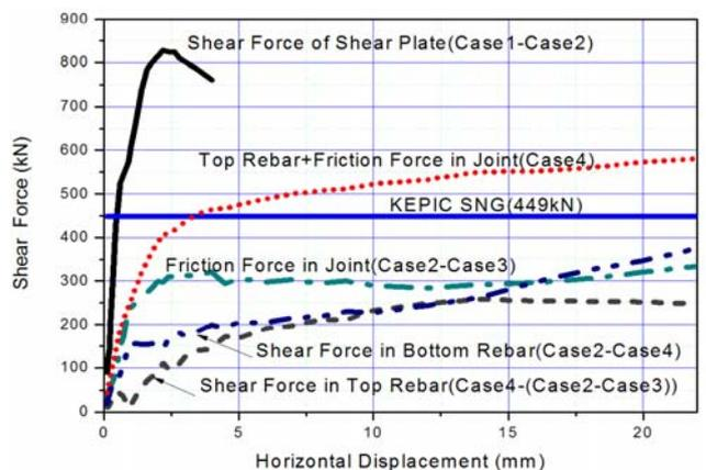
Fig. 27 Comparison results of shear force and KEPIC SNG
