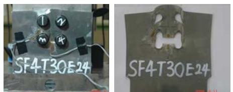
(a) at ultimate strength point / at test finishing point
