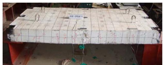
Fig. 5 Failure mode of No.0 specimen
