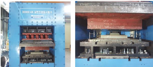
Fig. 2. Compressive test setup
