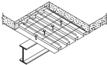
Fig. 1. Conventional H-shape composite beam
