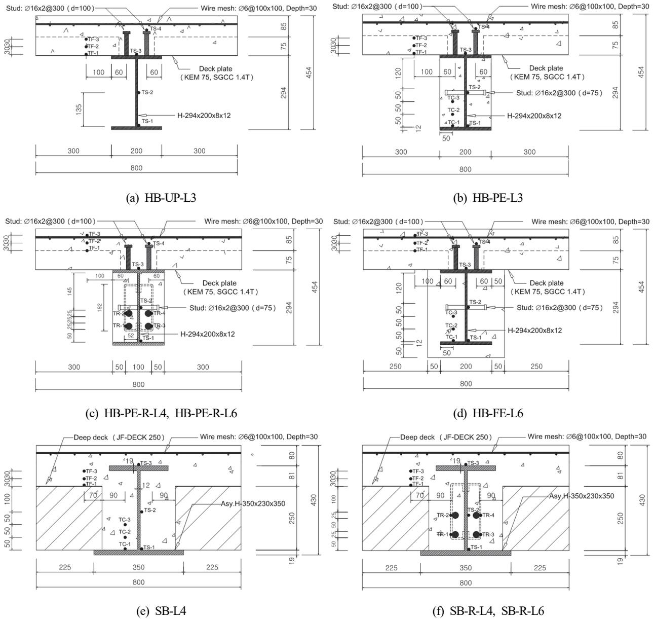
**Fig. 3.** Section details and location of thermocouples
