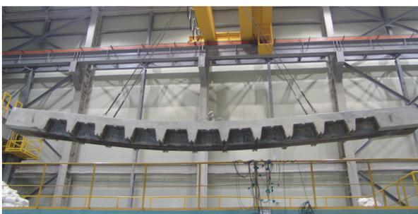
Fig. 7. Specimen after fire test
