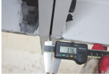
Gap of end-plate at tension side (end of loading)
