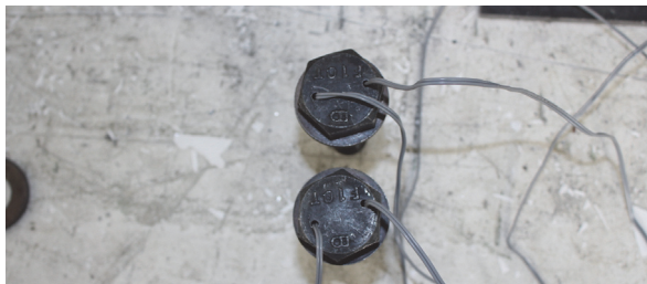
Fig. 8. Strain gauge install on H.T.B
