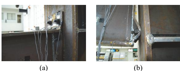
Fig. 5. Unstiffened end-plate connection experimental model (cycle 31)
