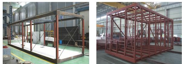
(a) Framed module (b) Load-bearing walled module
