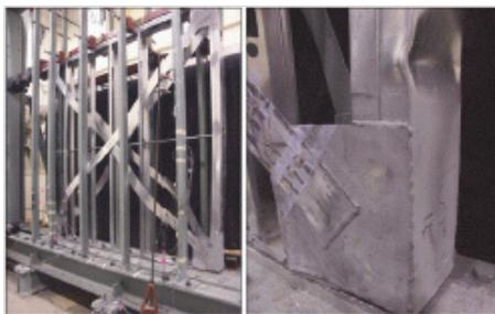
Fig. 2. Cold-formed strap-braced stud deformation and flexural failure of chord studs (M. Al-Kharat, C.A. Rogers, 2006)
