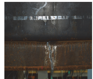
(b) ㄷ-Shaped bottom plate fracture
