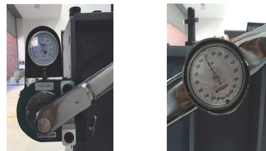
Fig. 5. Measuring the torque coefficient
