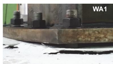
(b) Pull-out failure of concrete
