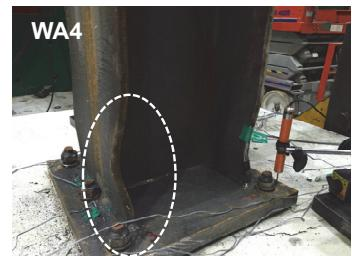
(c) Local buckling at beam flange section
