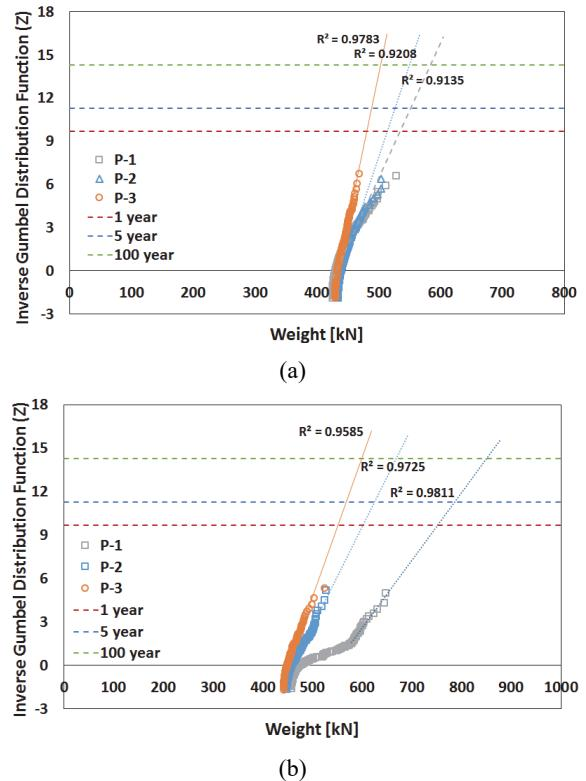
Fig. 2. Estimation of maximum weight of (a) CL 7 truck (b) CL 12 truck
