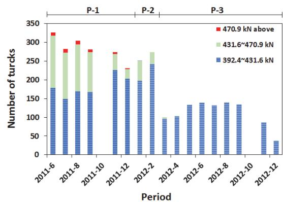
Fig. 1. Average number of daily truck traffic of class 7 and 12 over the legal restriction weight of 40ton (392.4kN) by month
