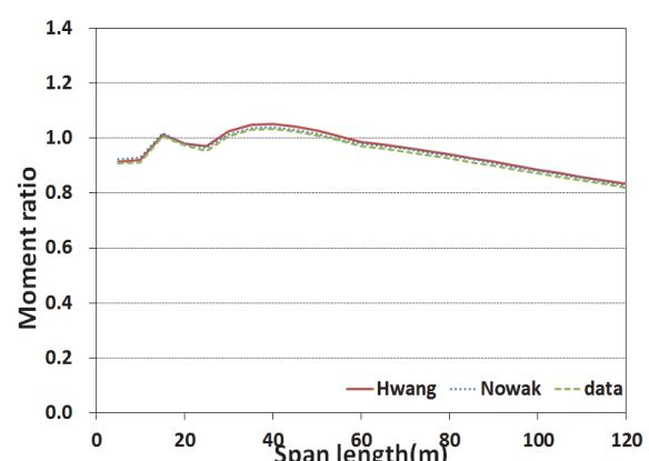
**Fig. 5.** Maximum moment envelop by two serial trucks
