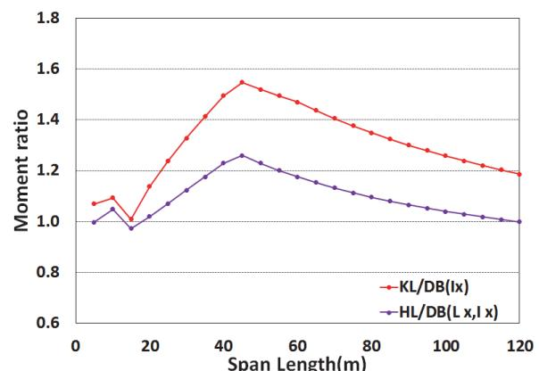
Fig. 11. Moment ratio of KL-510 and HL-93 to DB24
