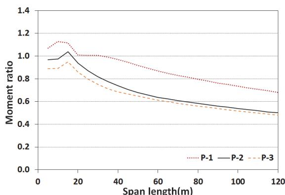
**Fig. 3.** Moment ratio of a single truck with maximum estimated weight to KL-510
