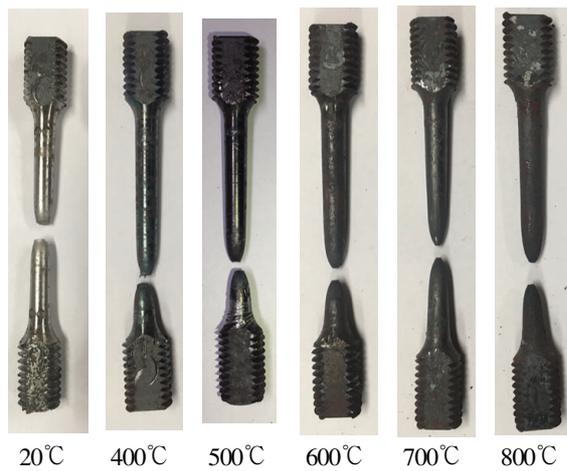
Fig. 5. Failure shape of SS275 at elevated temperature
