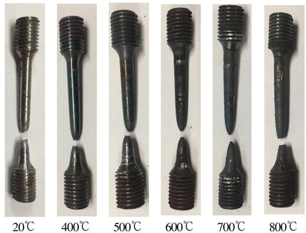
Fig. 7. Failure shape of SM355 at elevated temperature
