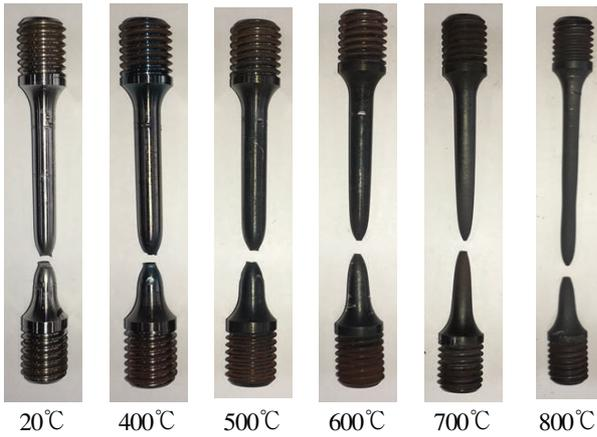
Fig. 9. Failure shape of F10T at elevated temperature
