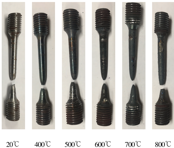
Fig. 8. Failure shape of SM355 (SM490) at elevated temperature
