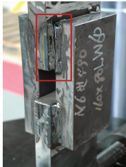
(a) Longitudinal welding specimen failure mode
