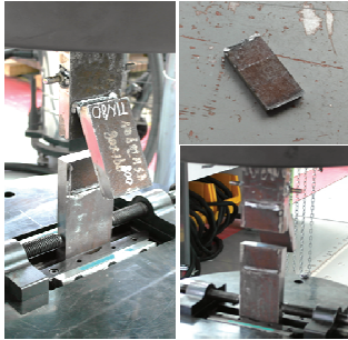
(c) TW800-1 specimen failure mode (extremely brittle rupture)
