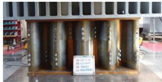
(a) Bolt failure
