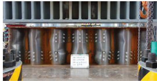
(a) Local buckling failure
