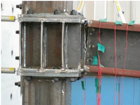
(b) Failure aspect of welded joints fracture at 0.04rad
