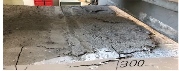
Fig. 10. Failure mode of slab
