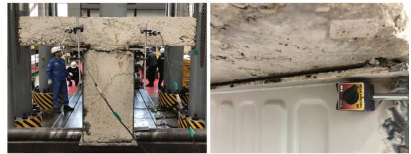
Fig. 12. Separation between steel and concrete
