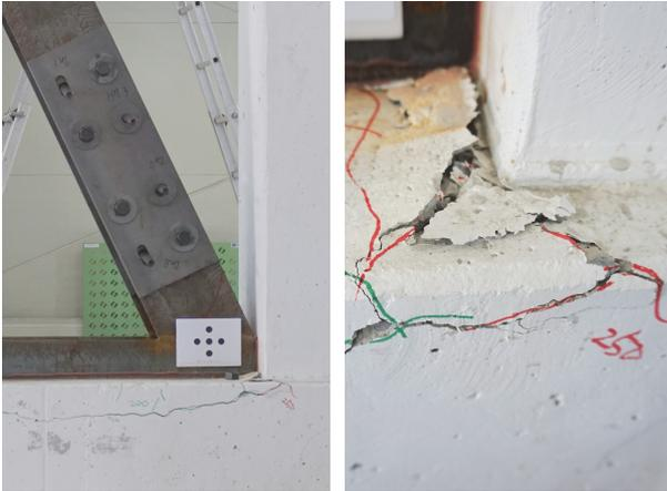
Fig. 21. Damage of NS-KF specimen
