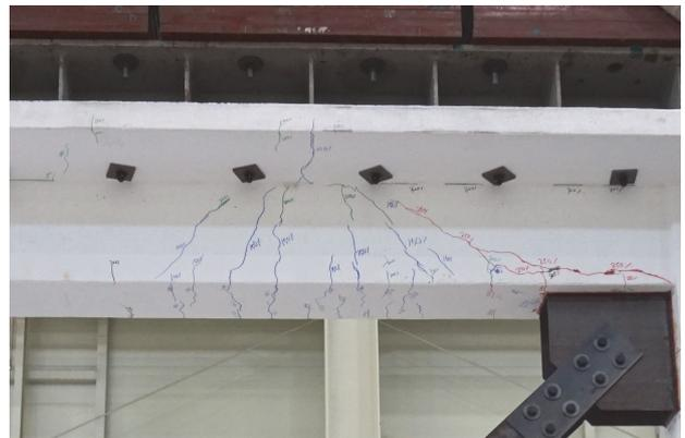
Fig. 20. Damage of NS-BF specimen
