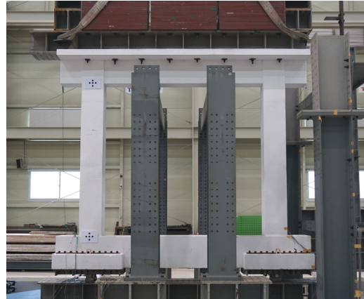
Fig. 3. Experimental setup for shaking table test (NS specimen)
