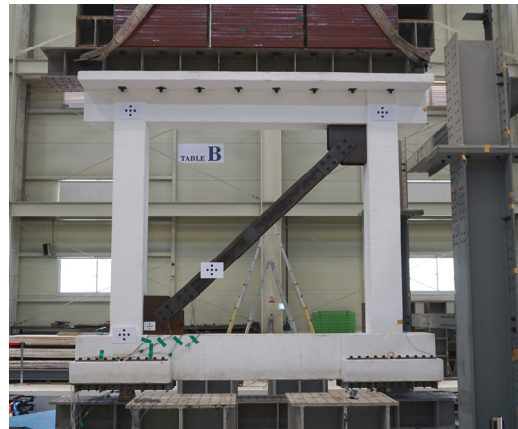
Fig. 4. Experimental setup for shaking table test (NS-BF specimen)
