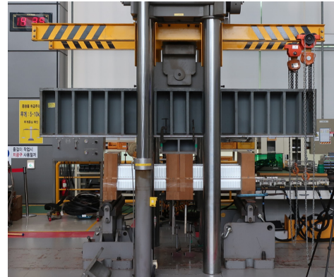
Fig. 7. Test set-up for shear test
