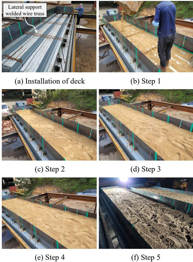
Fig. 4. Test procedure for sand loading test
