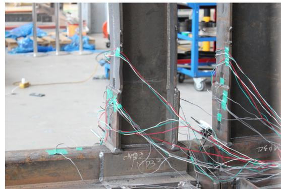
**Fig. 11.** Failure mode of BCHB2 at 4%
