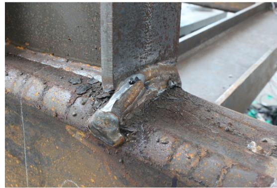
**Fig. 9.** Failure mode of BCHB1
