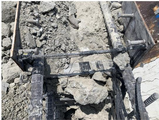
Fig. 6. Tie to prevent splitting of specimen no. 1
