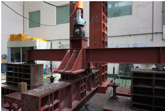
Fig. 7. Lateral bracing for ambient temperature
