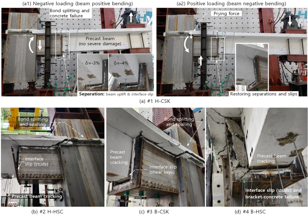
Fig. 9. Failure modes of precast composite beam-to-PSRC column connections
